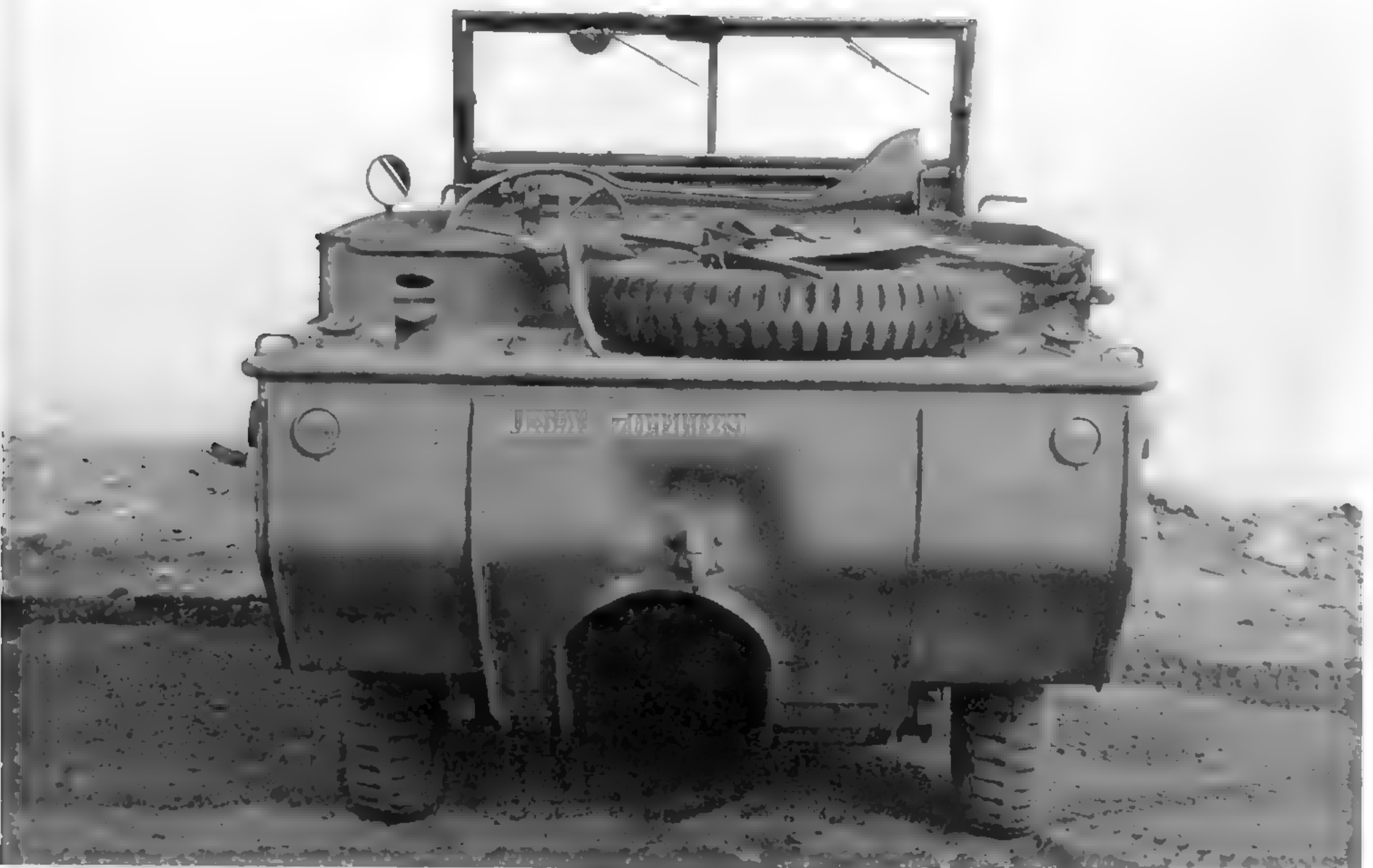
On the GPA, the Danforth anchor is stowed on top of the spare tire, the rifle rack is mounted on the windshield, and the offset tunnel houses the propeller and rudder. (U.S. Army photo)
